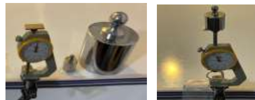
Fig. 8 Installation of clamp and gauge, weights and models (we used a neodymium magnet (1.3g) for more fixity of weights during measurement).
