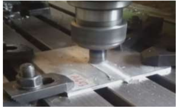
Fig. 3 Photograph of the process showing machine, tool and plate processed by FSP.
