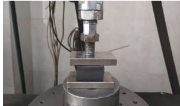
Fig. 8 The harmonic dynamics testing device at the moment of applying force on the elastomer.
