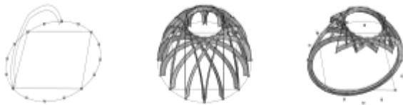
Fig. 4 Ring-like Karbandi structure created with specifications of a=b=4 , d=6 and using the first arch in "Fig. 3".
