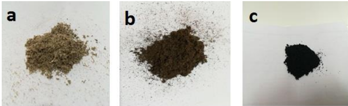
Fig. 1. Obtained hydrothermal carbon derived from the leather leaf at three different temperatures; a) 100, b) 150, and c) 200 °C
