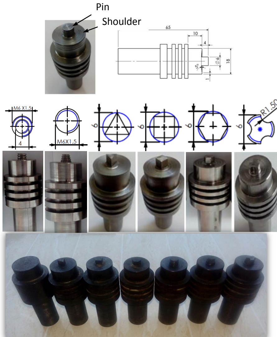
Fig. 1. FSW tools dimensions used in this study
