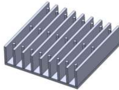
Fig. 7 Schematic diagram of square PFHS with pin angle of 22.5 degrees.
