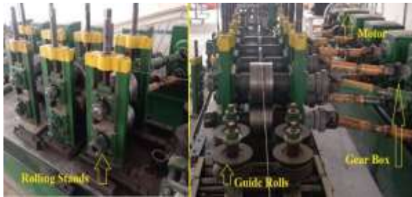
Fig. 4 Roll forming apparatus of the investigated machine.
