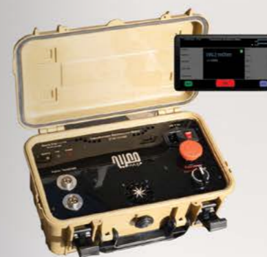
Transformer Resistance Meter
