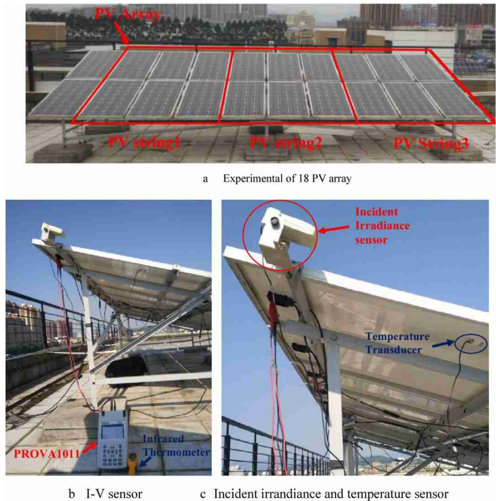
Fig. 4 Experimental platform. a Experimental of 18 PV array. b I–V sensor. c Incident irradiance and temperature sensor
