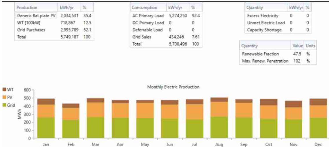
Fig. 7 Electric production from the grid-tied hybrid power system
