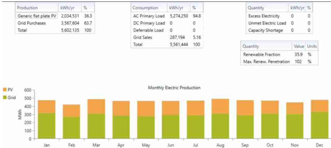
Fig. 10 Electric production from the grid-tied rooftop solar power system
