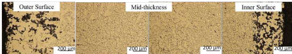
Fig. 4. Typical optical microscope images of the sample used after 45,000 hours of service.
