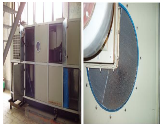
Figure 3. Photo of the solid adsorption cooling system equipment and wheel for doing experiments
